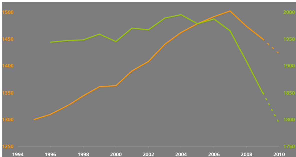
Figure 5: Development of curb weight (orange [kg]) and capacity (green [ccm]) new passenger cars(de Haan 2011).
