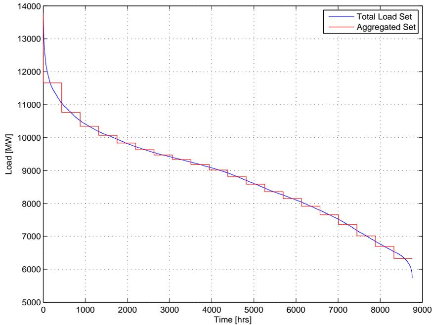
Figure 3.1: Load Duration Curve with Aggregated Set
