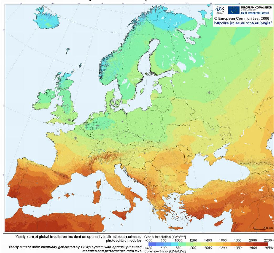
*Figure 5: Photovoltaic Solar Electricity Potential in European Countries. Incident radiation is high in red areas and low in blue areas.*
