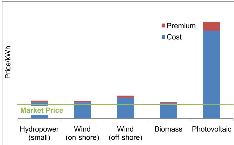
Figure 3: The principle of feed-in tariffs. The costs of renewable technologies exceed the market electricity price. A fixed tariff which covers both the cost and an additional premium is needed to make these technologies profitable.
