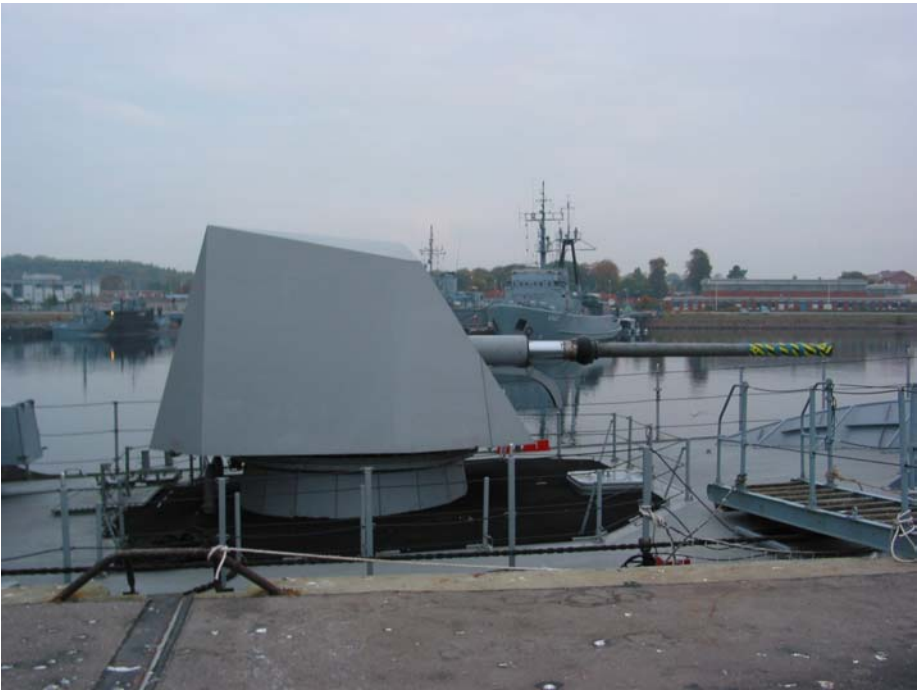
Figure 5: New 76 mm Gun with Stealth Cupola integrated by LÜRSEN.
