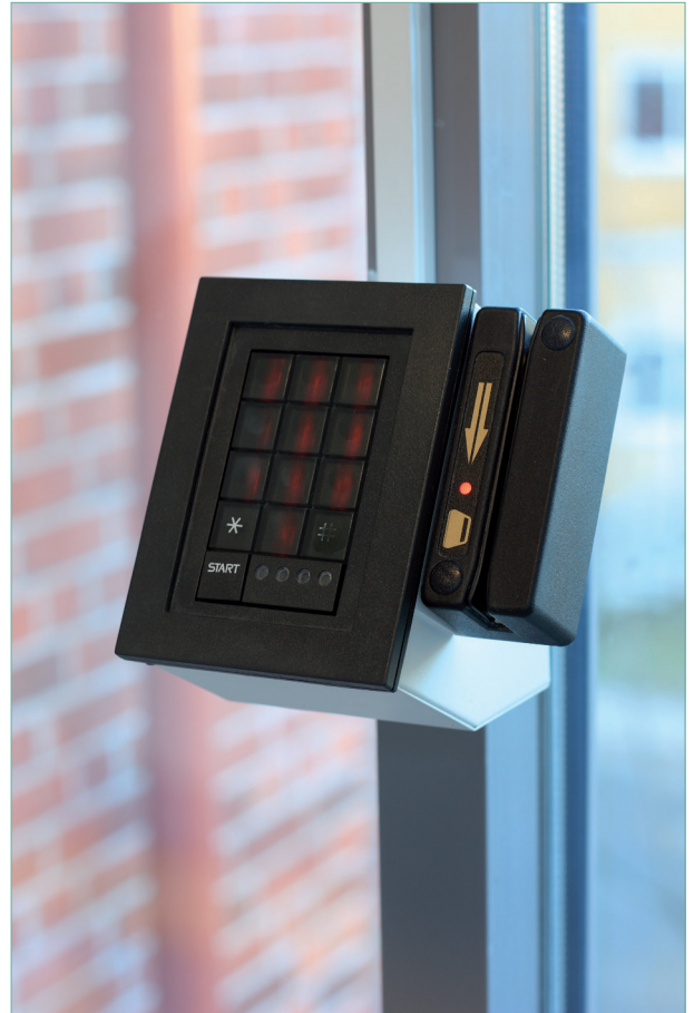
Electronic card reader with a scrambled numerical pad
