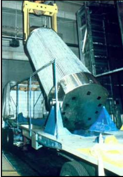
Figure 7.2 A typical small SNF shipping cask being mounted on a truck Courtesy of Nuclear Energy Institute
