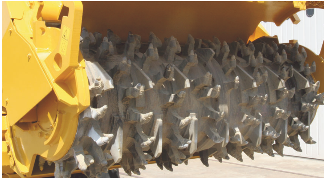
THE MINEBULL | Detail of the tiller system
