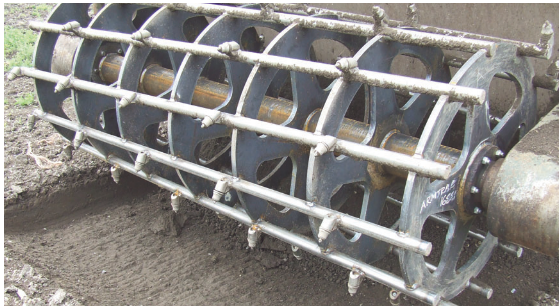
ARMTRAC 100 | Tiller stopped showing achieved depth
