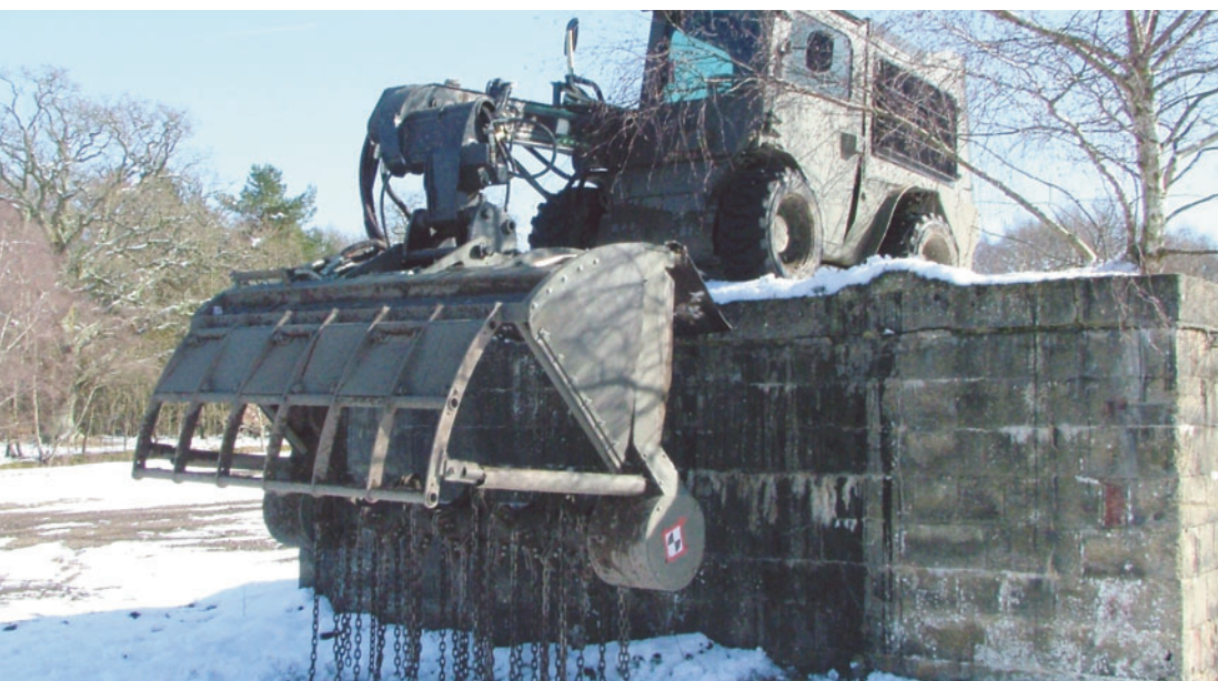
ARMTRAC 75 flail cleaning over ramp
