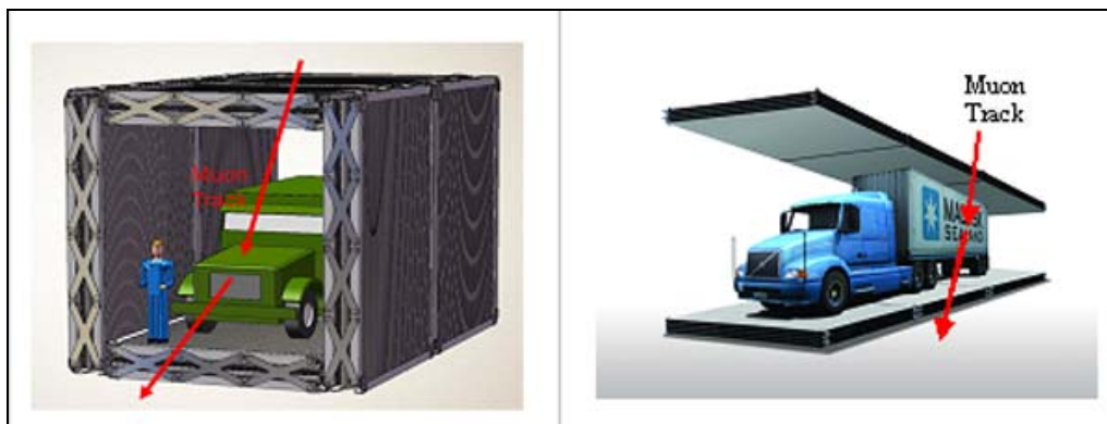
Figure 15. Schematic Drawing of Muon Tomography Inspection Station Configurations: Tunnel and Top/Bottom
