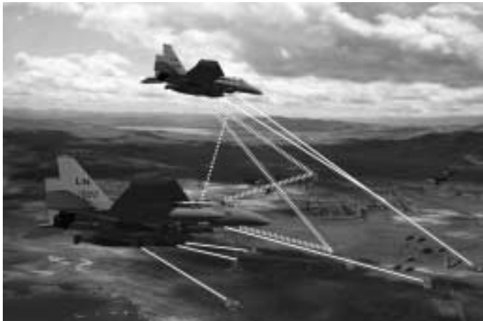
Figure 2. A pair of F-15Es locating radars. Each sees a portion of the threat array (solid lines) and, using data link (dotted line), performs cooperative ranging against the threats that are seen by both aircraft (dashed lines).
