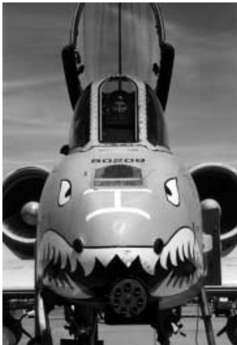
The A-10 Thunderbolt II's 30 mm GAU-8/A Gatling gun, which fires 3,900 rounds a minute, can defeat an array of ground targets, including tanks. Some of its other equipment includes an inertial navigation system, electronic countermeasures, target-penetration aids, self-protection systems, and AGM-65 Maverick and AIM-9 Sidewinder missiles.
