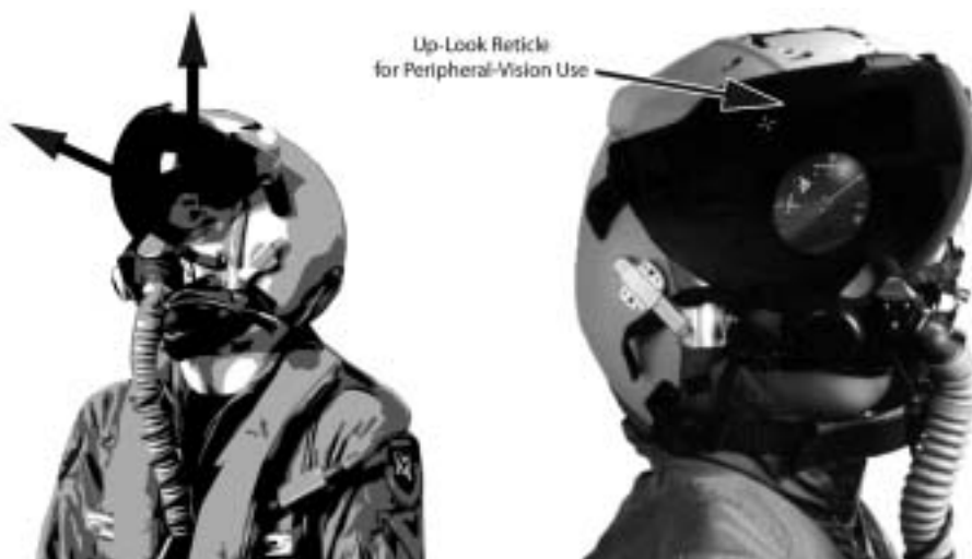
Figure 4. JHMCS peripheral-vision up-look reticle. (Reprinted from Maj Reid Cooley, briefing, subject: Joint Helmet-Mounted Cueing System, 422d Test and Evaluation Squadron, Nellis AFB, Nevada, June 2001.)
