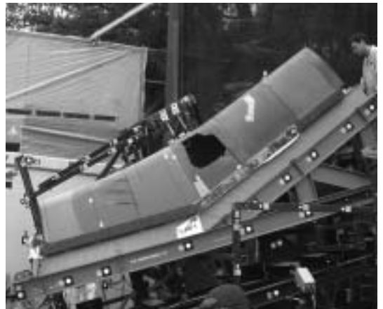
Foam can hurt. It was not until a 1.67-pound chunk of foam was propelled at 500 mph against an orbiter wing panel that naysayers in NASA came to realize that foam could indeed damage the leading edge. In this dramatic test, a piece of foam using the same impact conditions (foam type, size, weight, angle, and speed) that it would have had when it broke away from the bipod ramp and hit the Columbia , created a hole approximately 16 x 17 inches.
