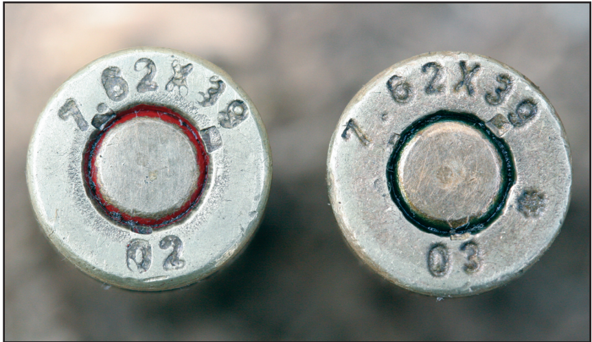
Figure 4 Comparison of headstamp marks
