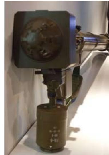
FN-6 with close up on Thermal Battery
