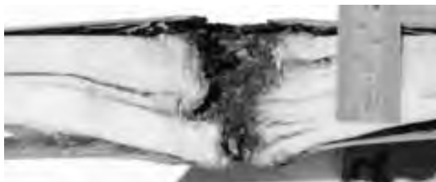
Figure 28: F6 – Dyneema Liner Deformation
