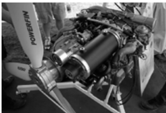
Figure 2. Flight Design’s hybrid-electric propulsion system. (Reprinted by permission from Jason Paur, “Hybrid Power Comes to Aviation,” Wired.com , 28 July 2009, http://www.wired.com/autopia/2009/07/hybrid-aviation .)
