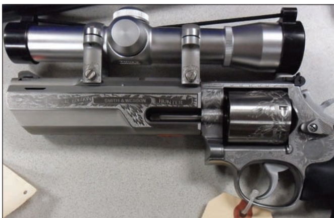
Figure 10 High-quality marks through mechanical engraving
