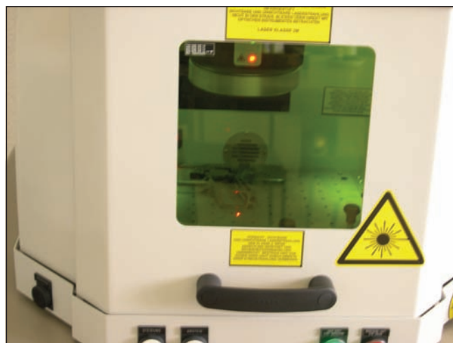
A standard laser machine can easily accommodate handguns and machine guns inside the safety cabinet. For larger arms, the laser machine may have to operate without the safety cabinet, requiring additional safety measures. Photos courtesy of GravoTech GmbH, Switzerland
