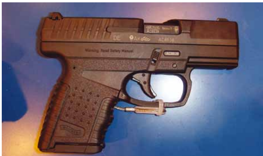
Polymer frames, increasingly used in firearms destined for the civilian market, present challenges in marking weapons durably. Photo: Robin Ballantyne / Omega Research Foundation
