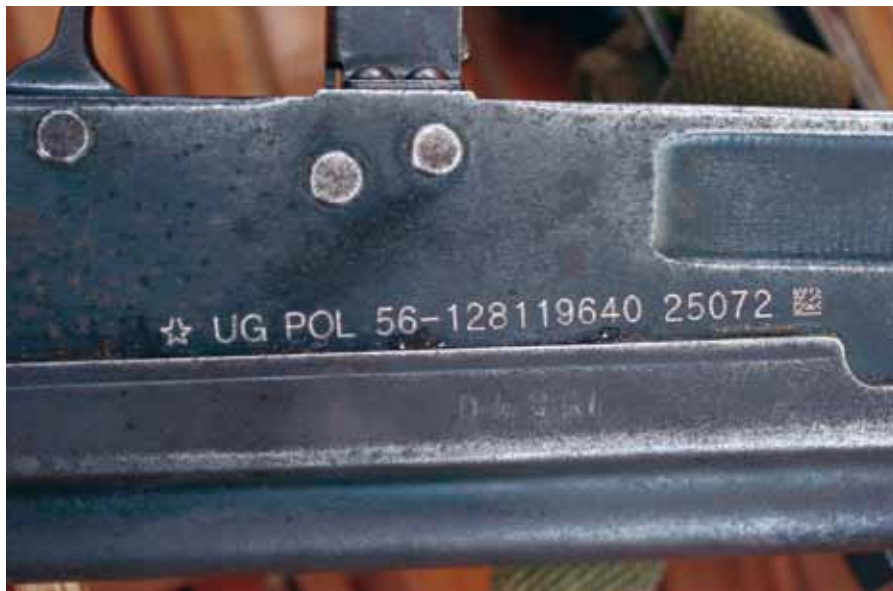
Ugandan police markings applied to a Chinese Type 56 assault rifle as part of Uganda's initiative to mark all small arms and light weapons in defence and security force inventories. Photo: Conflict Armament Research Ltd., 2012
