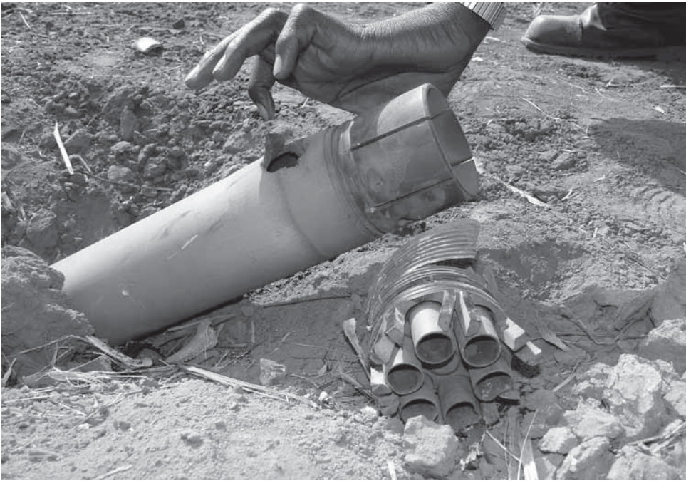
Fragments of 80 mm S8 air-to-ground rockets fired by SAF Su-25 aircraft next to an SPLA base, Firga, South Sudan, February 2011. © Confidential
