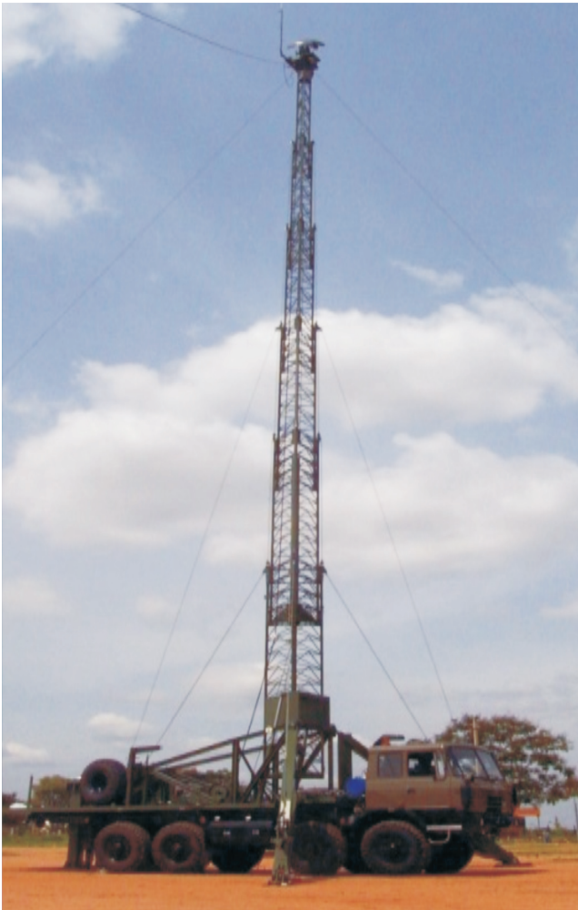
Mobile Battle Field Surveillance Radar
