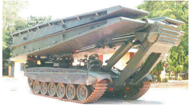
Bridge Layer Tank T-72
