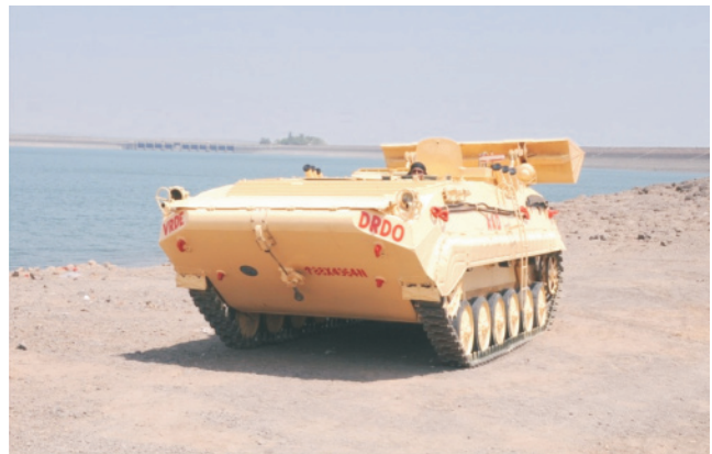
Armoured Amphibious Dozer (AAD)
