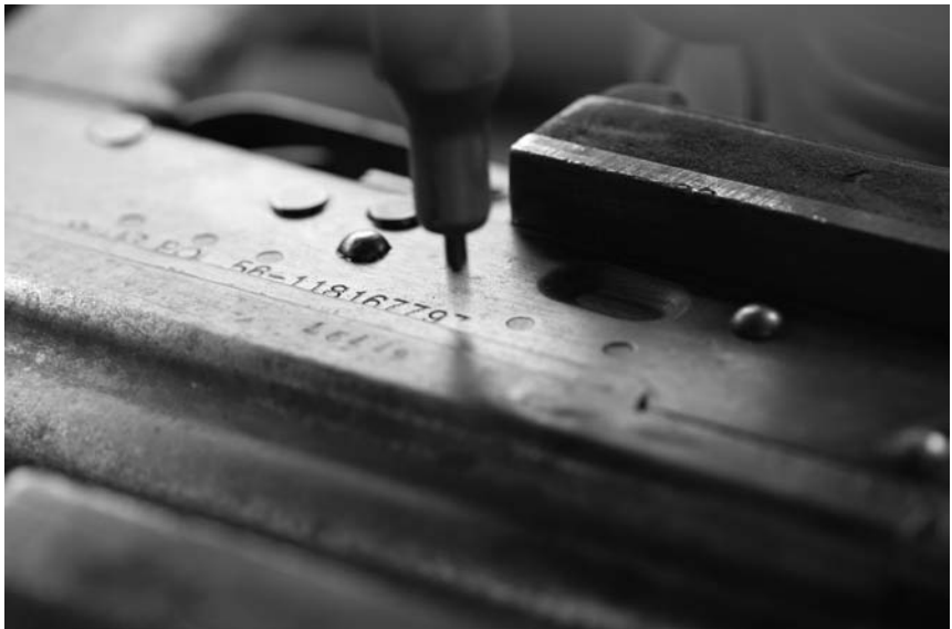
Figure 1 A dot-peen marking machine in operation
