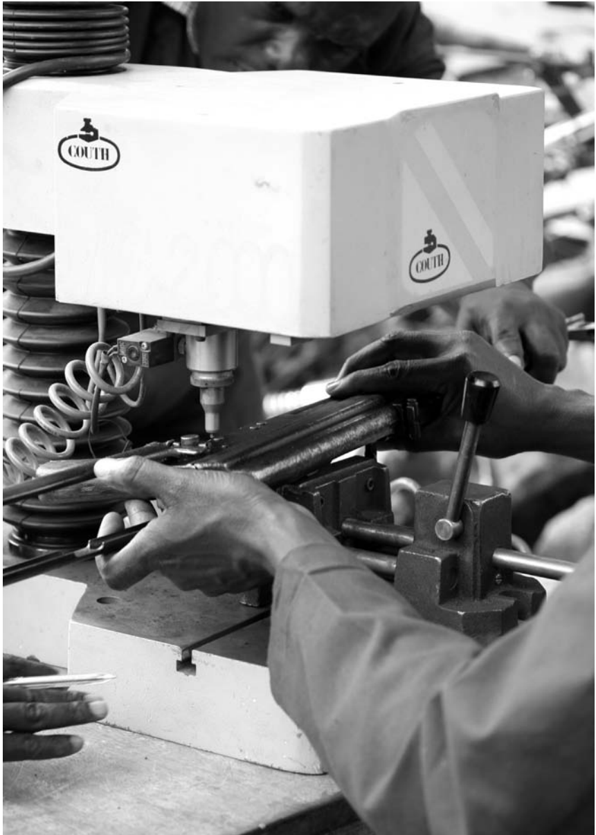
Figure 4 A Ugandan marking team seats a 1970s-era AKMS assault rifle in the Couth MC 2000 marking machine
