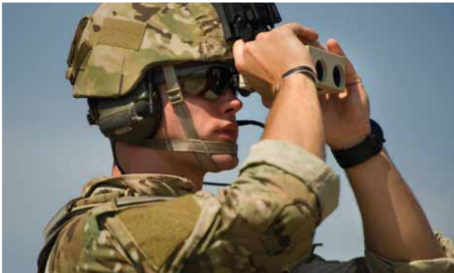
A Fire Support Officer from the Army's 75th Ranger Regiment identifies targets for air strikes using a laser rangefinder during a training exercise.
