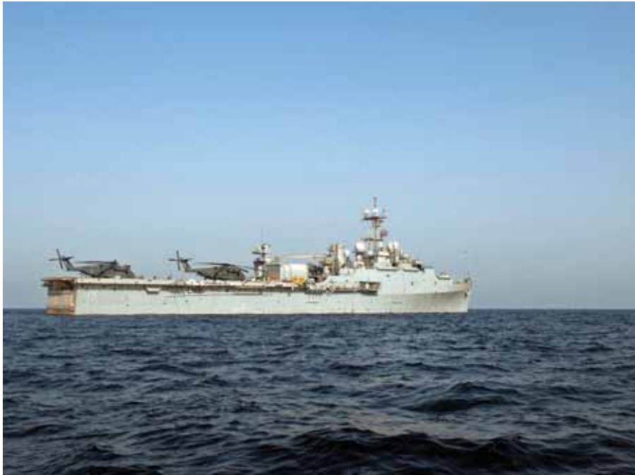
The Navy recently retrofitted the USS Ponce as an Afloat Forward Staging Base. With its well deck and large landing surface for rotary-wing aircraft, the Ponce could be an effective sea-base to support special operations ashore in austere or inhospitable environments.
