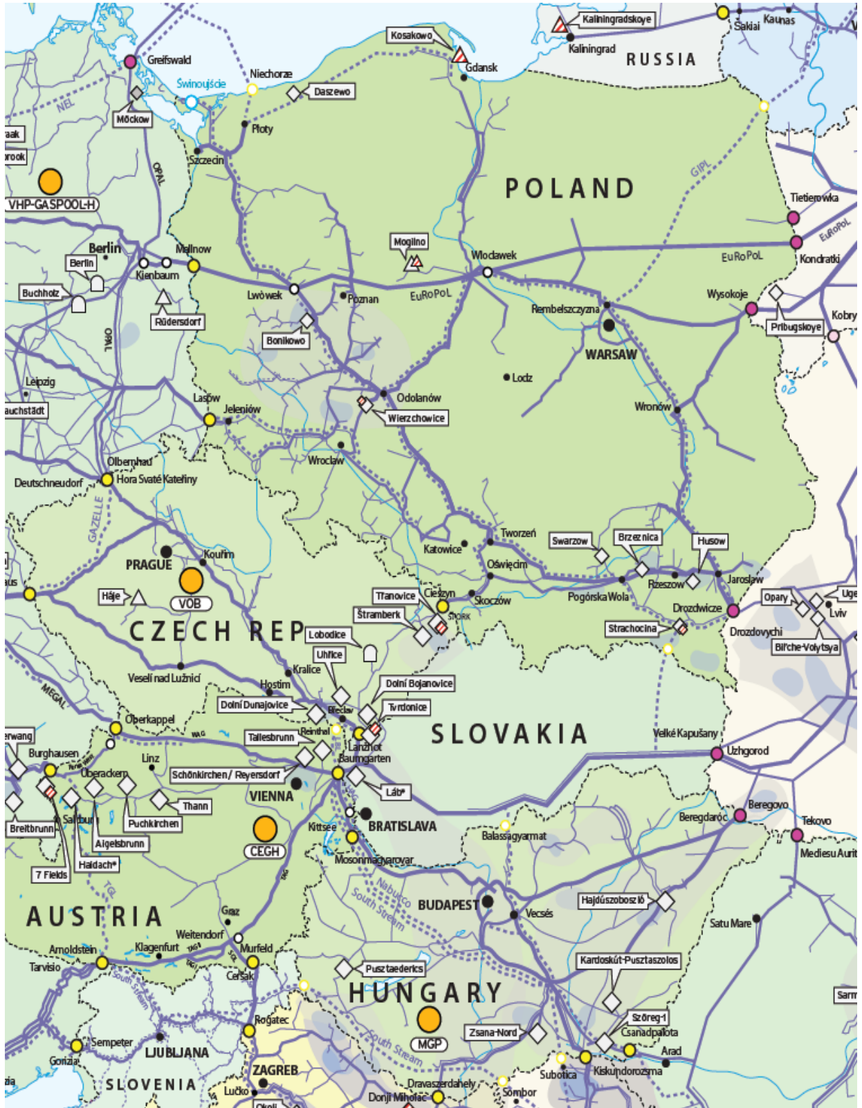
Figure 1. Transmission pipelines in V4 and neighbouring countries (source: ENTSOG/GIE: dotted lines are planned).
