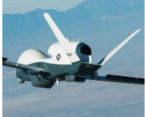
The U.S. Navy Triton is specially designed to fly surveillance missions up to 24 hours at altitudes of more than 10 miles, allowing coverage out to 2,000 nautical miles.
