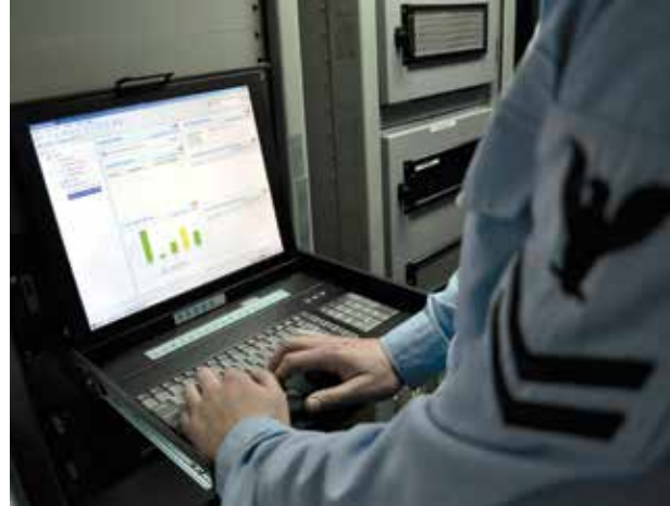
Petty Officer 2nd Class Ryan Allshouse uses the intrusion detection system to monitor unclassified network activity from the automated data processing workspace aboard the aircraft carrier USS Ronald Reagan . IDS is part of the integrated shipboard network system and serves as an important computer network defense enabler protecting the unclassified shipboard network from cyber attack.
