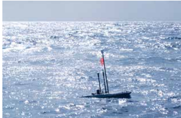
Wave-powered uninhabited surface vessel.
