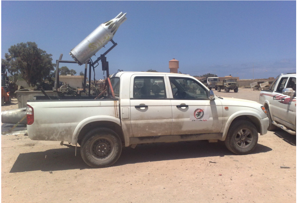
Photo 18 UB-16-57 launcher mounted on a pickup truck in Libya, in 2011.
