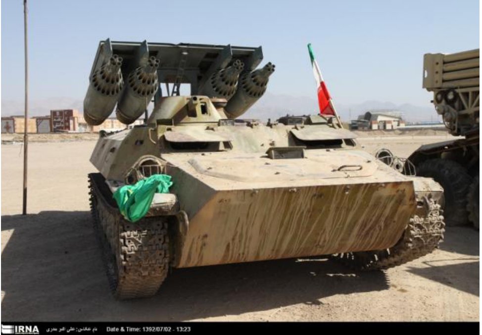
Photo 6 A captured Iraqi MT-LB retrofitted with four UB-32-57 rocket pods on display in Iran.
