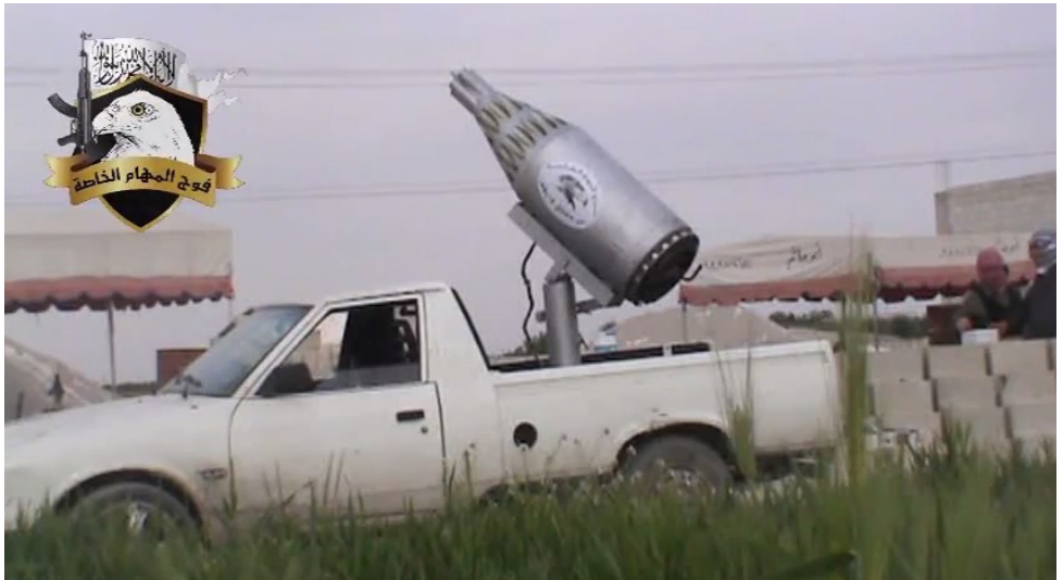
Photo 22 UB-32-57 launcher mounted on a pickup truck of one of the Syrian armed opposition groups.
