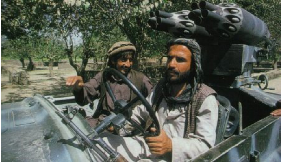
Photo 14 and 15 Improvised rocket systems based on UB-16-57 launchers in Afghanistan in the late 1990s or early 2000s.
