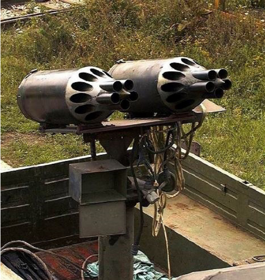
Photos 8 and 9 A TAM-110 truck operated by Republika Srpska forces in Bosnia and Herzegovina in the mid-1990s, fitted with two UB-16-57 rocket pods. Photo credit: UK Ministry of Defence
