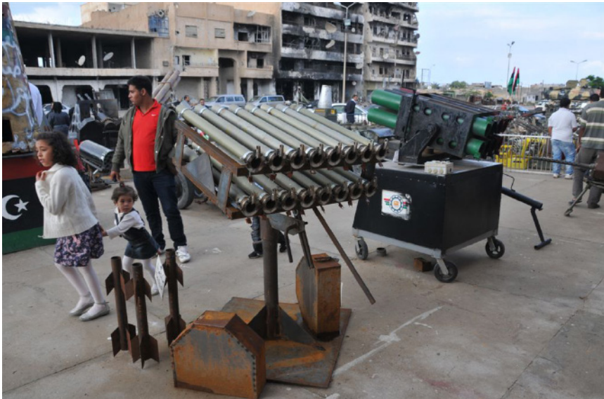
Photo 21 Improvised sixteen-tube rocket launcher for 57 mm S-5 rockets in Libya. Photo credit: Vadim Naninets
