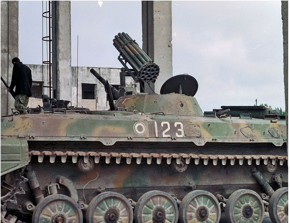
Photo 12 A Georgian Army BMP-1 AFV with a stripped-down UB-16 type rocket launcher. This particular improvised system was described as being employed in an anti-helicopter role.
