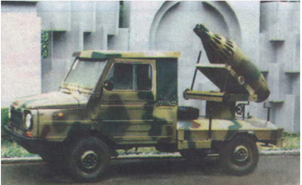
Photo 25 Ukrainian prototype MLRS vehicle based on a LuAZ-969M truck with UB-32-57 rocket pod. Pictured in 1998. Photo credit: Monetchikov, 1998
