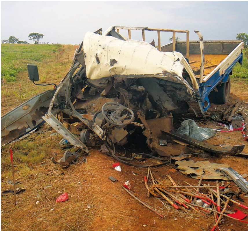
| Truck damaged by AVM explosion in Angola.
