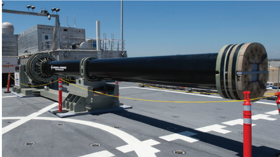
FIGURE 11. THE 32-MJ EMRG BARREL ON USNS MILLINOCKET (JHSV-3)
