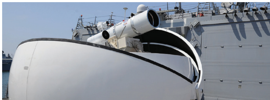
FIGURE 10. LASER WEAPONS SYSTEM DEPLOYED ON USS PONCE
