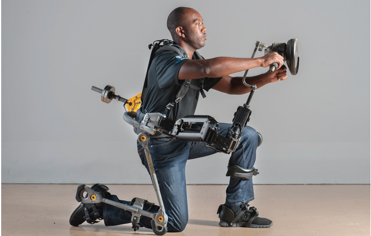
FORTIS exoskeleton with the user holding a heavy grinding tool. (LOCKHEED MARTIN)
