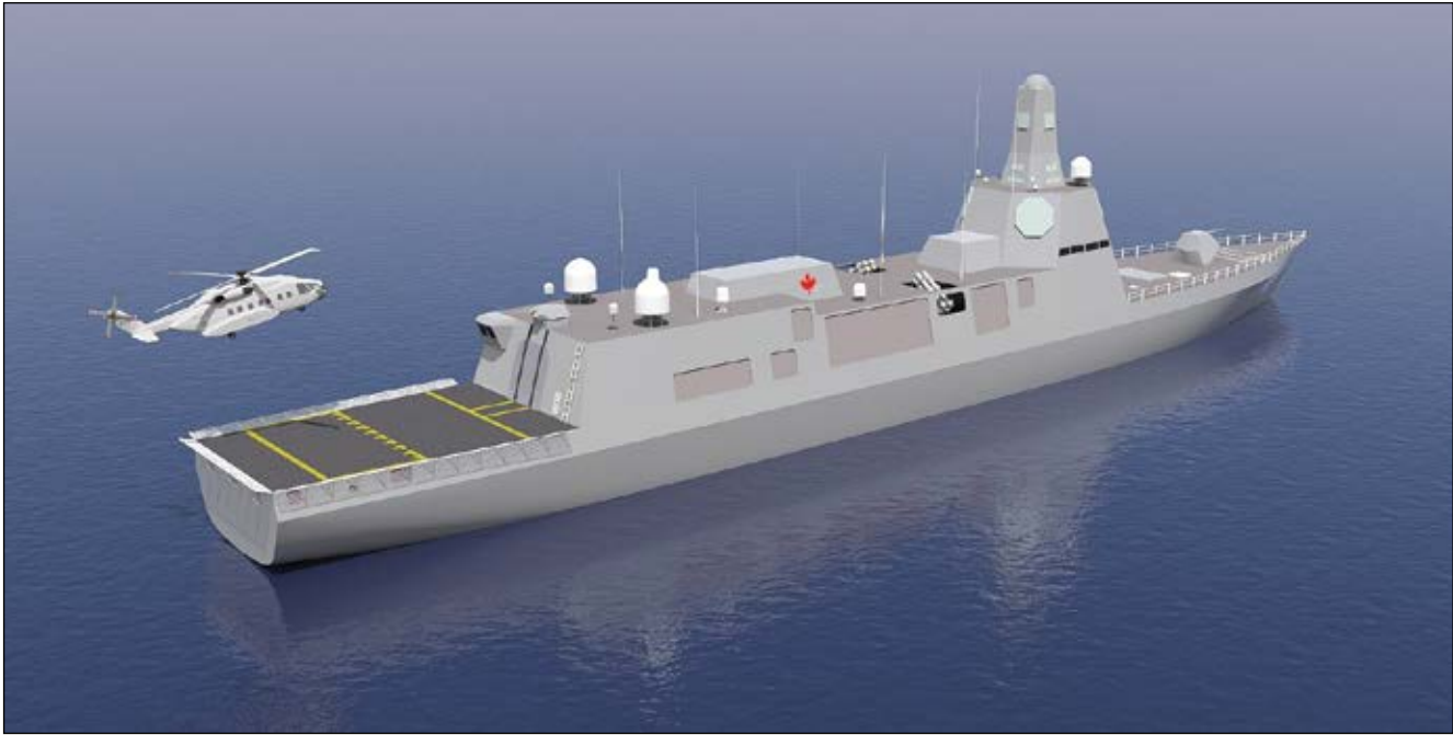
Rendering of a concept design of the Canadian Surface Combatant Ship. On 20 January 2015, the federal government announced that Irving Shipbuilding in Halifax will be the prime contractor on the 15-ship Canadian surface combatant program.
