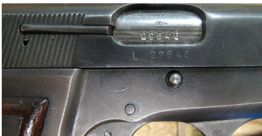
Figure 3b Weapon markings on a Belgian FN Herstal Browning Hi-Power self-loading pistol. Visible markings include the serial number (in two locations), the calibre, and proof marks. Source: N.R. Jenzen-Jones/ARES
