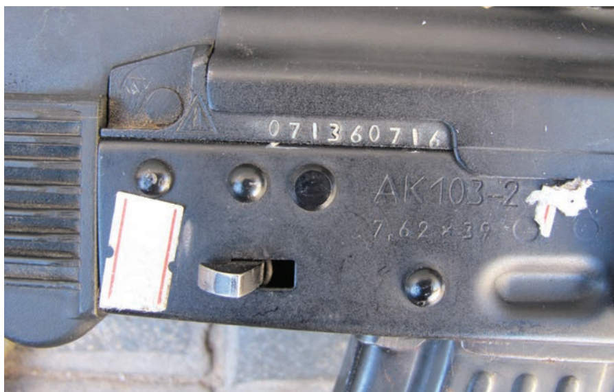
Figure 3a Weapon markings on a Russian AK-103-2 self-loading rifle. Visible markings include the manufacturer marking, serial number, model designation, and calibre. Source: Damien Spleeters
