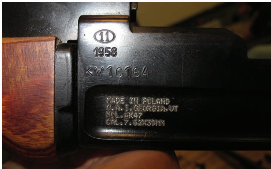
Figure 3d Import markings (showing country of origin, importing party, model, and calibre) on a Polish Kbk AKM self-loading rifle imported into the United States. Also visible are factory, year of production, and serial number markings. Note that the import markings on this weapon misidentify it as an ‘AK47’. Source: N.R. Jenzen-Jones/ARES
