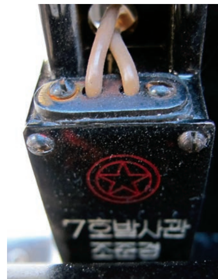
Figure 8a Markings on a North Korean copy of a PG0-7B optical sight. Source: Damien Spleeters
