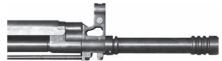
Figure 2b A spigot muzzle attachment, designed to allow the launch of rifle grenades.
