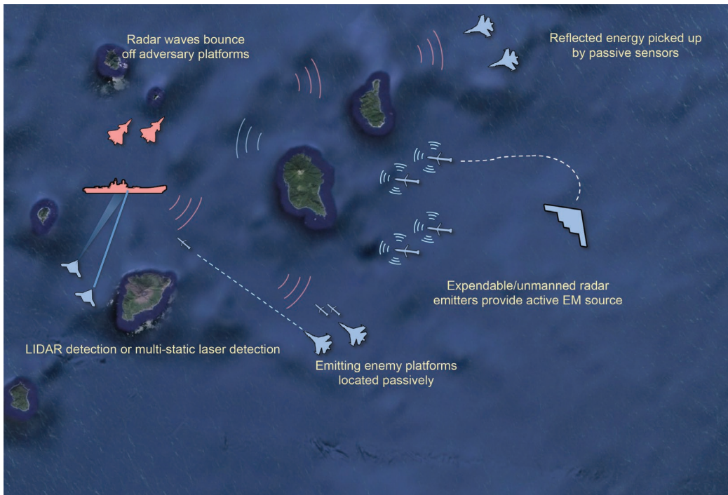
FIGURE 10. CONCEPTS FOR PASSIVE AND MULTI-STATIC DETECTION
