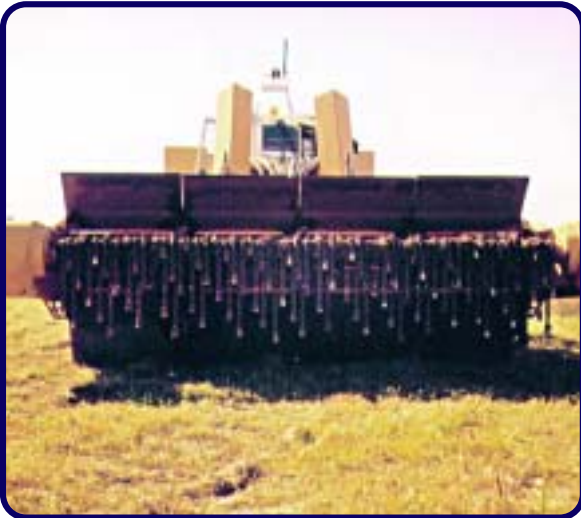
Figure 2 The flail unit chains and hammers
