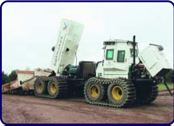
Figure 2 Scanjack with armoured hoods open
