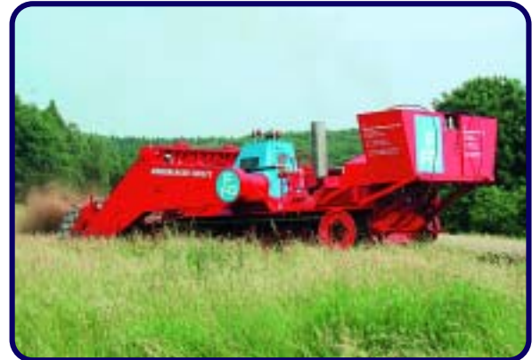
Figure 3 Minebreaker 2000/2 operating in open ground
