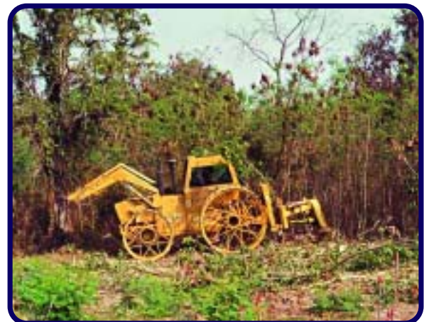
Figure 5 The Pearson Slasher at the rear of the tractor cutting vegetation
