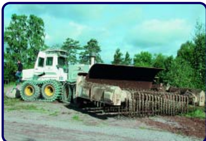
Figure 4 Scanjack 3500 with the articulated engine and flail unit
