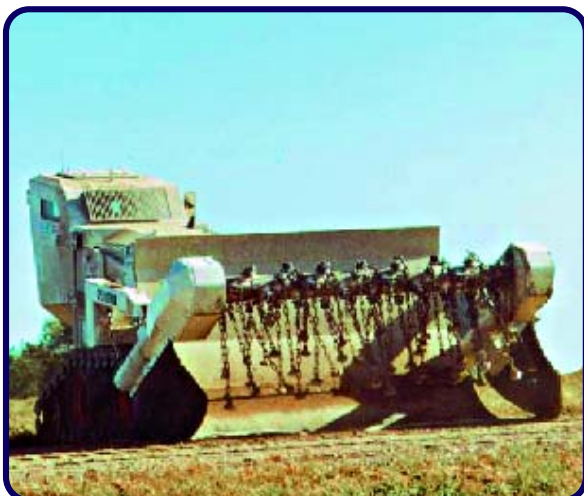
Figure 2 The flail unit of the Minecat 230
