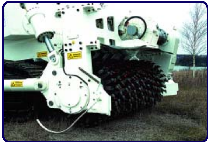
Figure 2 Roller with circular plates fitted with tungsten carbide teeth
