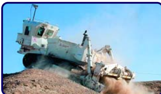
Figure 4 Mine-Guzzler clearing in Egypt
