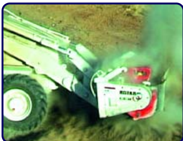
Figure 2 Mine blast within the Rotar drum
