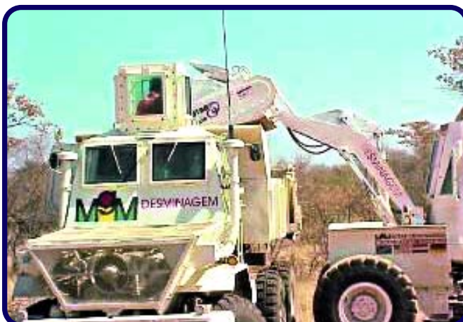
Figure 4 Rotar-I emptying suspect debris into a tipper
