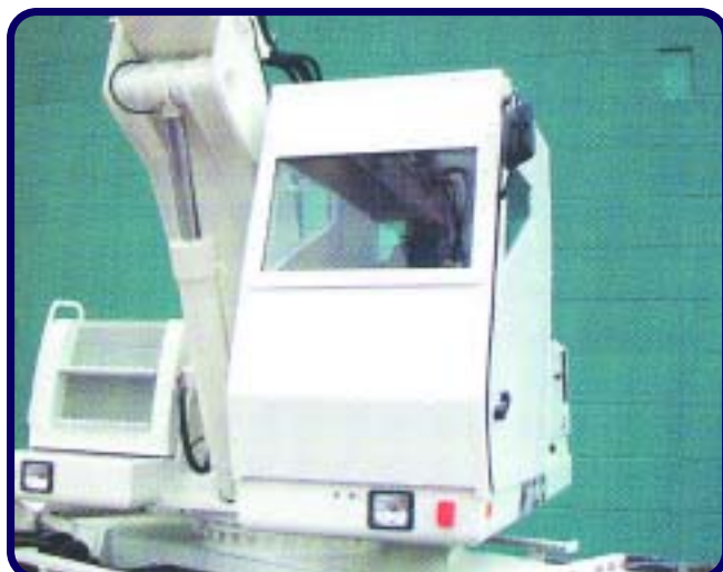
Figure 3 The armoured cab of Hydrema MI220
