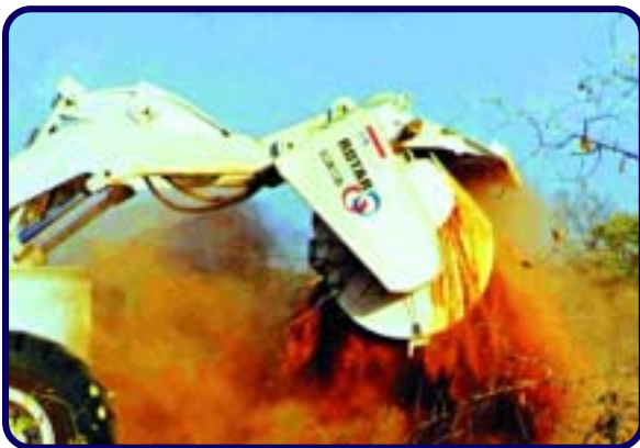
Figure 2 The Rotar sifting dry soil
