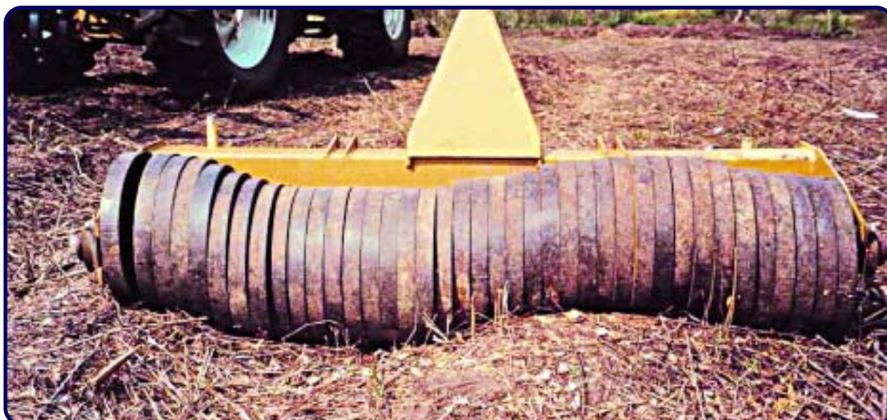
Figure 2 The area reduction roller with its 50 kg discs
