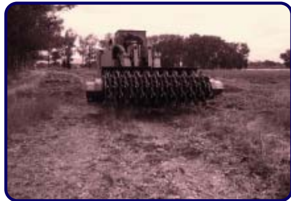
Figure 2 Spitfire tiller unit with carbide metal cutting bits
