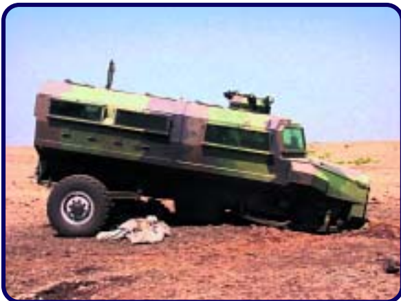
Figure 3 Wer'wolf after detonation of 14 kg TNT under the front axle
