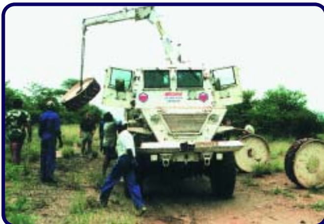
Figure 4 Early version of Casspir mounting steel wheels
