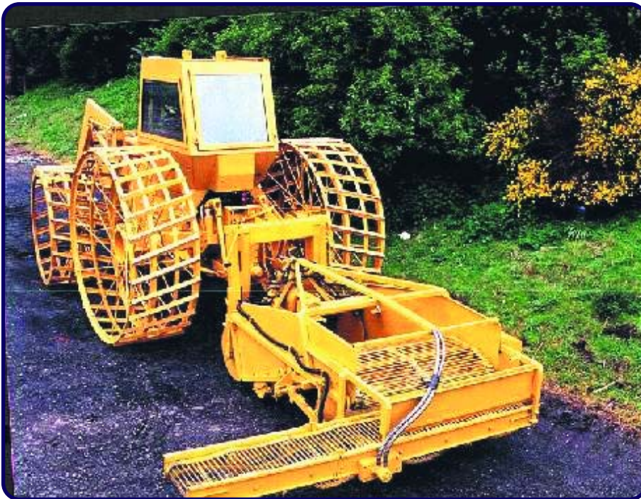
Figure 4 The Pearson Sifter fitted to the rear of the SDT
