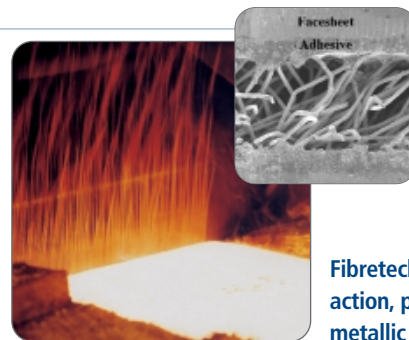
The structure of the metal 'sandwich'
