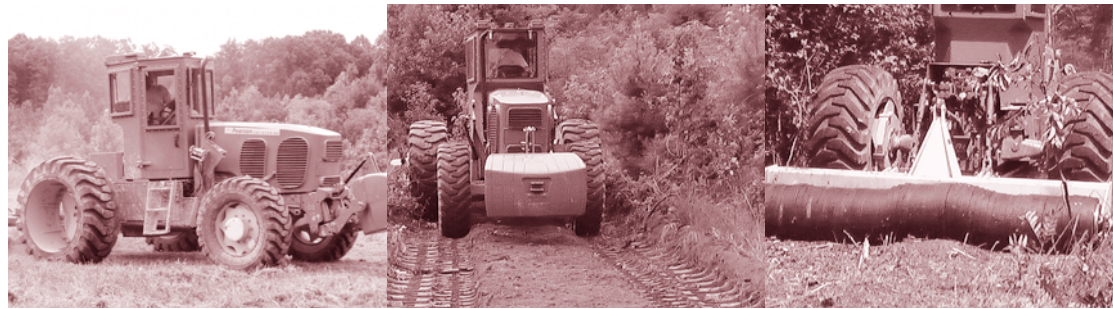
THE PEARSON MINEFIELD TRACTOR | Mine comb in heavy vegetation | Area reduction roller
