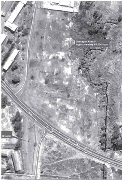
b) Photo interpretation of an IKONOS image (27 June 2005) for damage assessment
