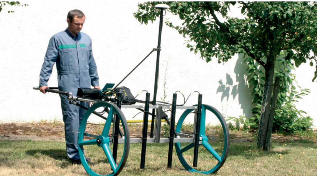
3 sensors mounted at vehicle
