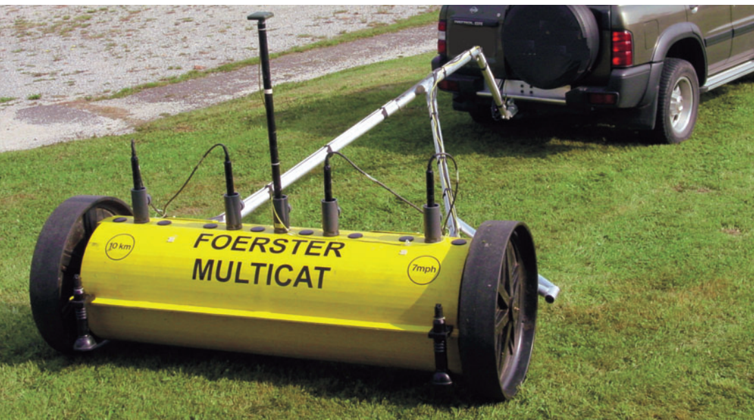
The MULTICAT equipped with four FEREX probes and GPS antenna
