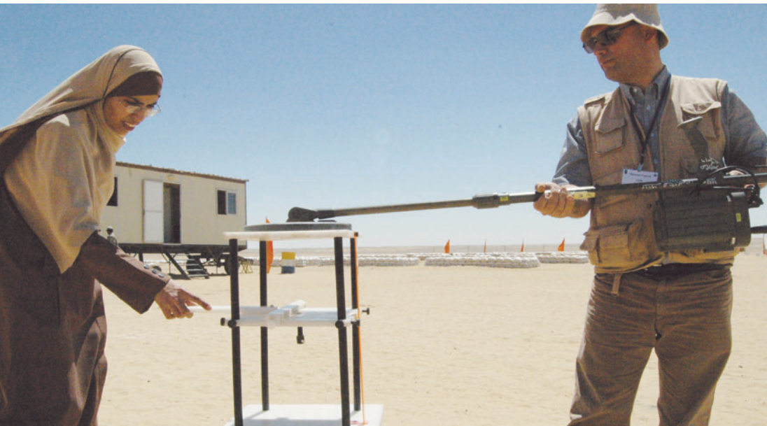
CEIA-MIL-D1 in use at the Egyptian test site: measurement of "in air reference height"
