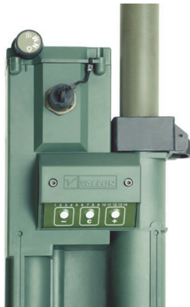
Sensitivity-, control-, and ground compensation push buttons with LED bargraph on the front of the housing
