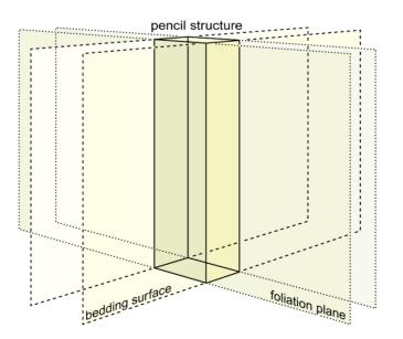
Intersection lineations and pencil structures are often utilized to determine the orientation of the unexposed, related fold axes.
