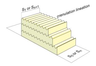
Rolling of some minerals during deformation may produce a wrinkling of an existing part of the foliation. If carried out far enough, this may produce some kind of chevron folds parallel to the rotation axis of the minerals, the resulting crumples trending across the general direction of flow.
