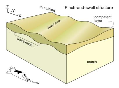
Pinch-and-swell and pull-apart structures may be combined at any level since they depend on the ductility contrast between the strong bed and its matrix.
