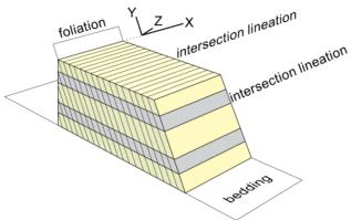
Two non-parallel foliations can also produce an intersection lineation; for example, the intersection of a crenulation cleavage and the earlier foliation. The more planar surfaces there are in an exposure, the more potential intersections there will be.
