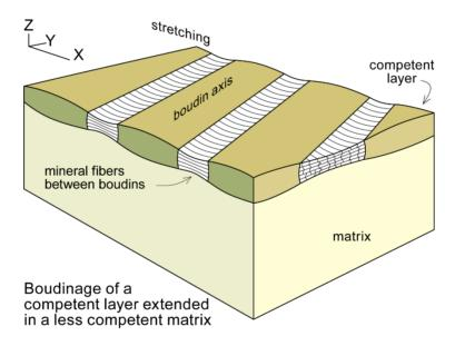
Boudin profiles are variable, symmetrical or asymmetrical. Long faces, usually layer boundaries of the boudins, can be concave (bone-shaped boudins), convex (barrel-shaped boudins) or parallel to each other (blocky boudins). These shapes reflect ductility contrasts between layer and matrix. Large contrasts produce boudins with sharp edges, and small contrasts produce rounded boudins.
