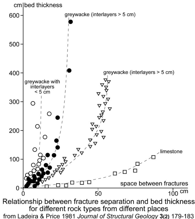
However, systematic investigations have shown that the thickness of incompetent interlayers influences fracture separation within competent layers. Spacing is wider where interlayers are thicker than a critical value assessed to be ca 5 cm; conversely, fractures are closer to each other where weak interlayers are thinner than 5 cm.
