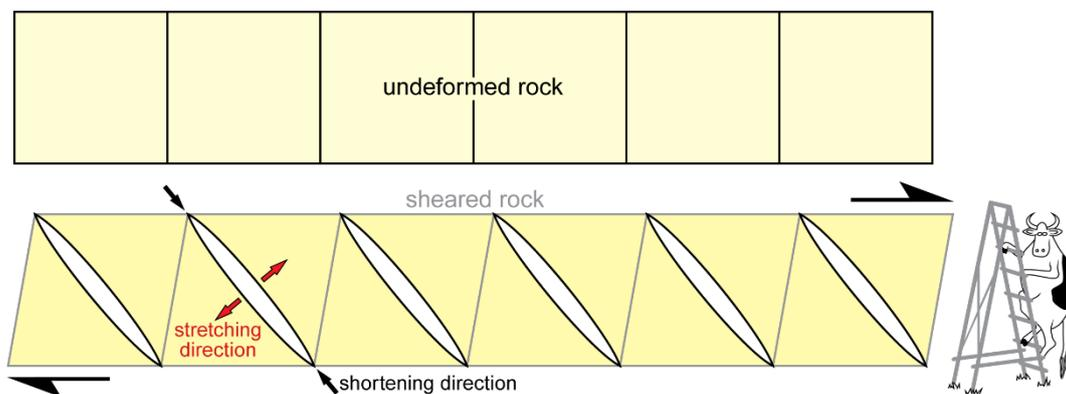
Development of *en échelon* tension gash array in a brittle shear zone (instantaneous stretching and shortening directions do not rotate during shearing)
