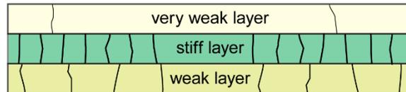
Spacing of bedding-parallel joints according to competence (elastic modulus) of layers
