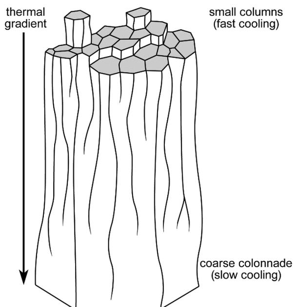
Sketched coarsening of a columnar joint pattern
