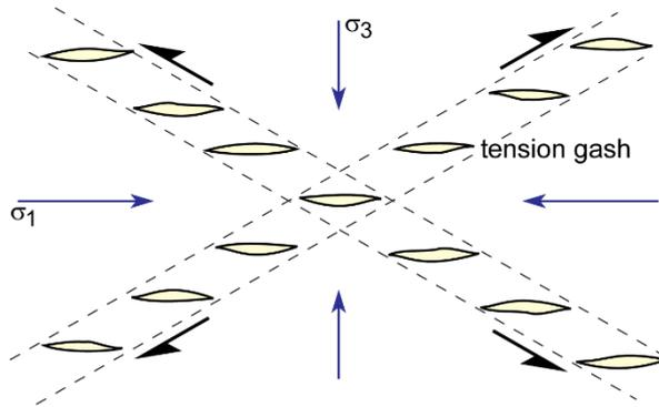
*En échelon* array of tension gashes along conjugate, brittle shear zones and sigmoidal gashes due to heterogeneous rotation of gashes in these shear zones
