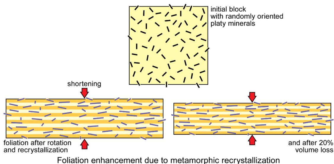
In some metamorphic rocks, the orientation of new crystals may be governed by, and is parallel to, the orientation of pre-existing grains or aggregates. Their shape fabric **mimics** the older fabric and sometimes inherits the shape of previous crystals, so defining a **mimetic foliation**. Growth is **mimetic**.
