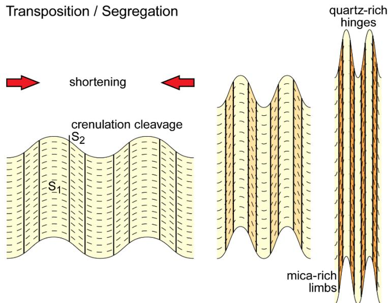
Metamorphic segregation in gneiss is important either by enhancing a deformational layering or by forming a new layering by pressure solution for example in the case of melt production.
