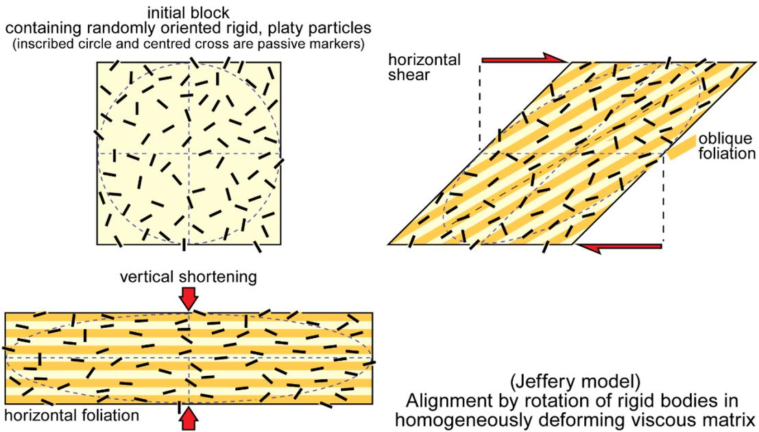
The progressively developed preferred orientations predicted by both, Jeffery and March models are essentially the same, Jeffery's analysis differing from that of March by a factor that describes the shape of the rotating particles. Furthermore, the Jeffery rigid particles define in simple shear regime a stable statistical orientation that cannot be achieved in the March model.
