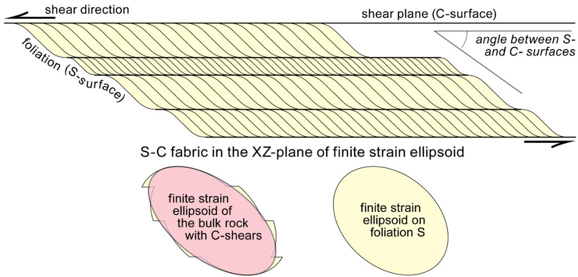
Each C shear zone is relatively planar and develops its curved foliation pattern on a small scale so that the sense of deflection of S into C is the same as the general sense of shear.
