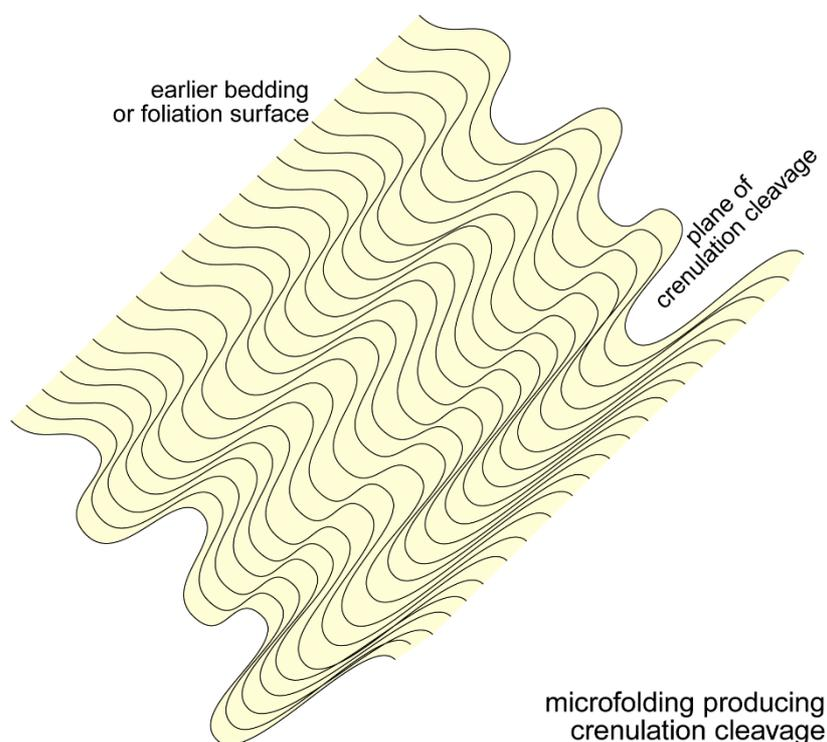
As the microfolds become more closely compressed, the limbs become progressively thinned out and parallel while the fold hinges become relatively thicker. The new crenulation cleavage is parallel to the aligned limbs of stacked microfolds. Micas within the limbs of crenulations remain approximately parallel to the earlier fabric. They are still parallel to the earlier foliation but have been rotated toward parallelism with the new foliation.
