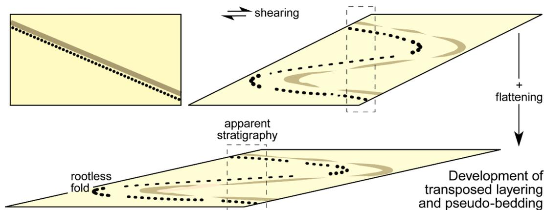
Fold hinges are sharp and folds are **intrafolial**. Hinges may be torn apart along the stretched limbs that ultimately disappear. The intrafolial folds are **rootless** where hinges are completely detached
