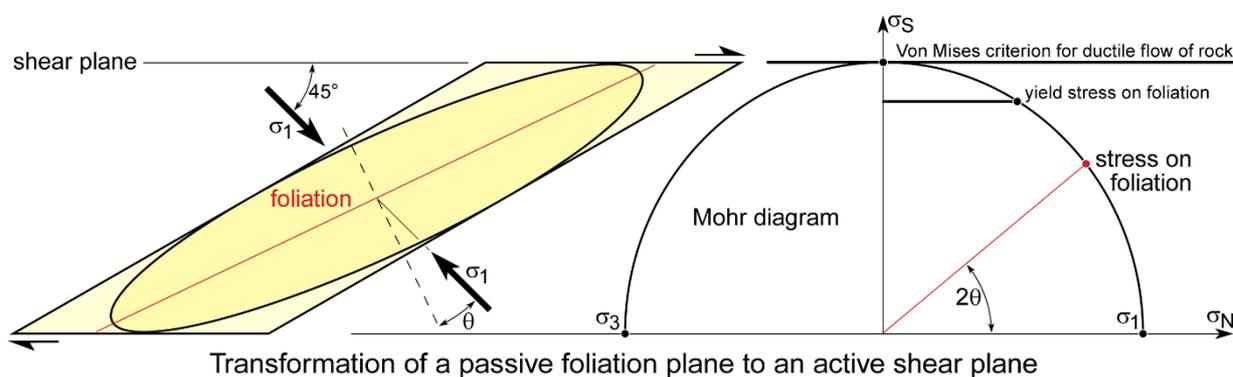
Transformation of a passive foliation plane to an active shear plane
