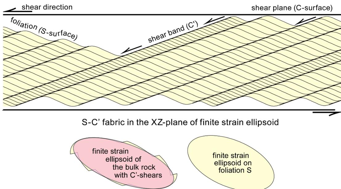
These micro shear zones are usually less continuous than C planes and delineate an extensional crenulation cleavage termed **C' planes**. S-C'-structures may indicate intense, non-coaxial and partitioned flow. Conjugate sets may arise to accommodate extreme flattening.
