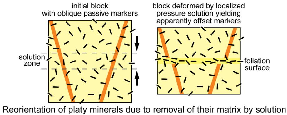
The juxtaposition of quartz-rich domains and cleavage domains with insoluble and densely-packed minerals suggests that pressure solution is involved in the formation of most foliation types.
