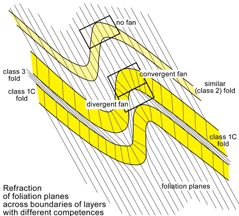
Due to fanning foliations, convergent and divergent foliation orientations form triangular regions with no cleavage in hinge regions of the less competent layers of folds: **the finite neutral points**.
