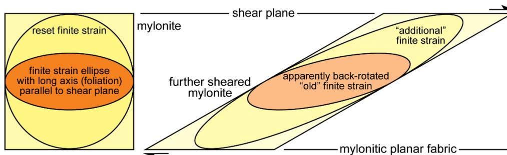
Instability of the finite strain ellipsoid in mylonites
