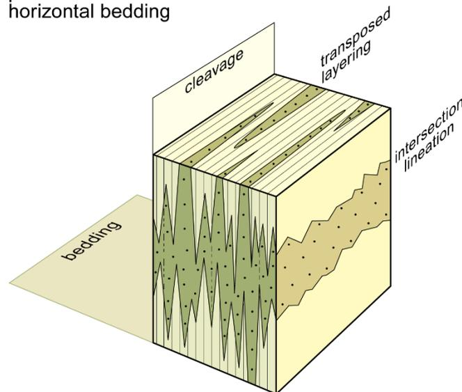
In a laminated sequence of rocks, successive layers generally have different competences. Intense deformation produces appressed to isoclinal folds through rotation and stretching/thinning of limbs until these coincide with the foliation plane.
