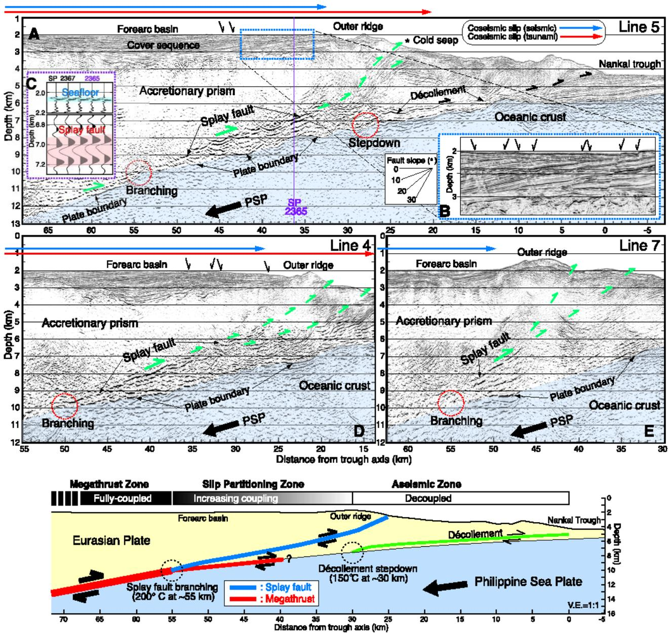
Depth migrated profiles of the Nankai subduction zone with sketched section interpreting seismic distribution and behaviour in the inner and outer parts of the accretionary wedge. From Park *et al.* 2002 *Science* 297(5584) 1157-1160.
