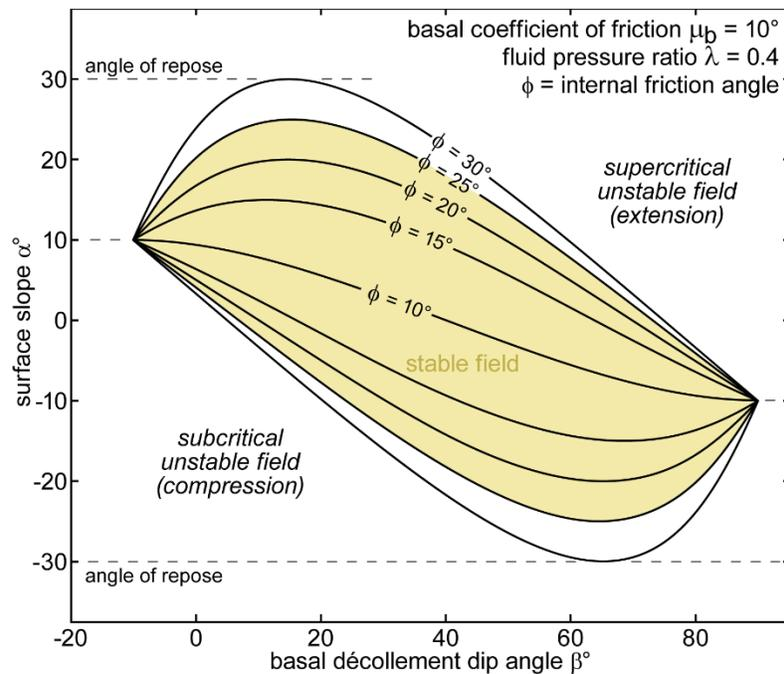
Two antisymmetric curves enclose a central area, which contains the surface slope angle and basal friction combinations for which the wedge remains stable, i.e., endures no internal plastic deformation. Outside the stability domain, the wedge is super- or subcritical.
