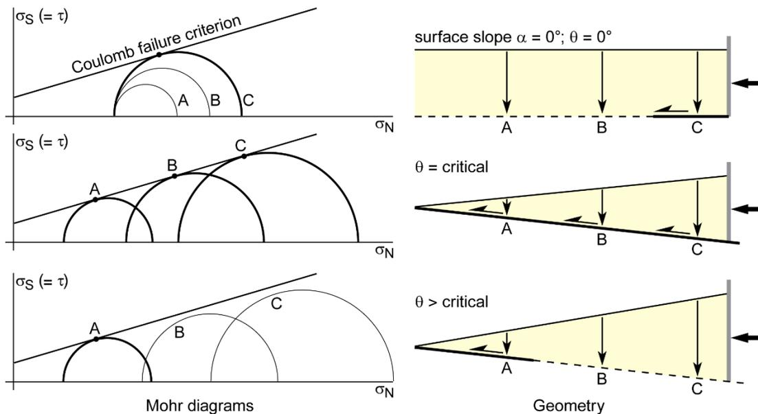
Conceptual representation of thrusting location according to the critical taper
