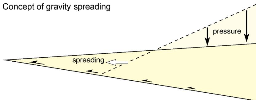
Shortening at the front of the spreading sheet balances collapse-related extension in the hinterland. Again gravity is the driving force. The topographic slope rather than the dip of the basal décollement is the geometric control for thrust movement. In addition, spreading forces continuously diminish while the
