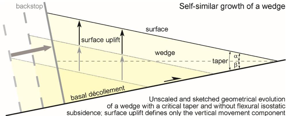
The analogy links the topography of orogenic belts to the rheology of the crust and includes the effects of body forces and externally applied tectonic forces.
